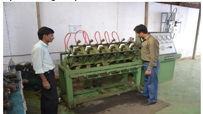
Hydraulic Hydro Testing Setup – Forged Valves
