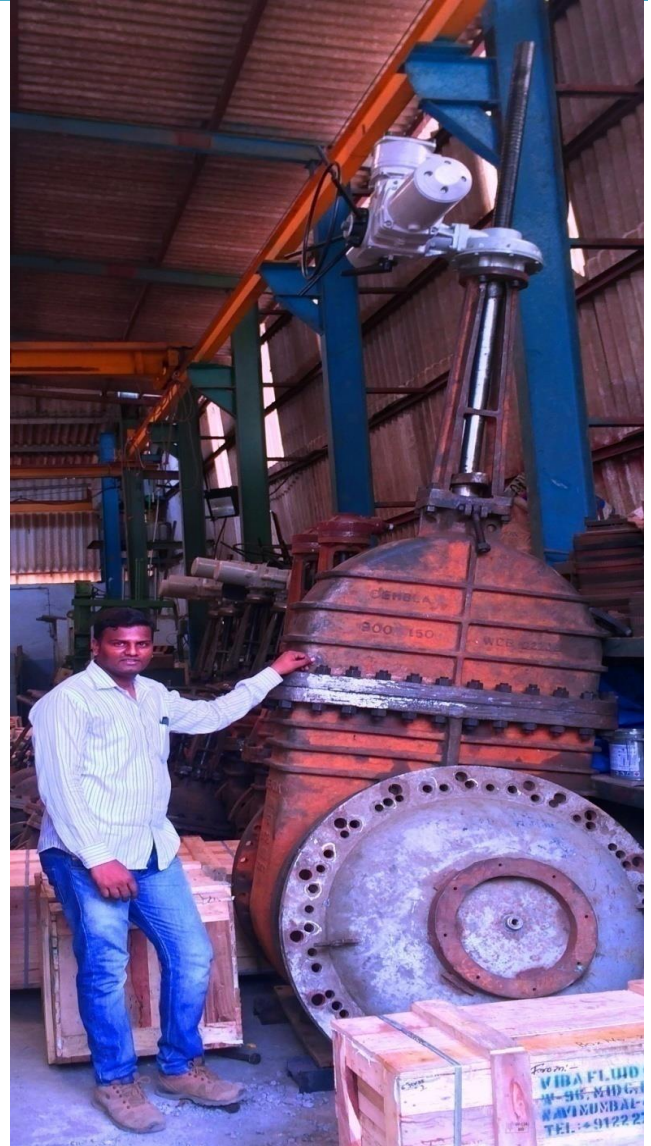
36" Cast Carbon Steel ASTM A216 Gr. WCB Gate Valve, Flanged Ends, Class 150 Supplied to Jindal Project
