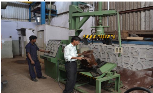
Hydraulic Hydro Testing Setup – Cast Steel Valves
